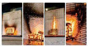
Poland's first LARGE SCALE TEST of exterior walls of buildings according to BS 8414-1:2020-04 "Fire performance of external cladding systems. Part 1. Test method for non-loadbearing external cladding systems applied to the masonry face of a building".
